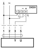
Control with 4...20 mA via external resistor
